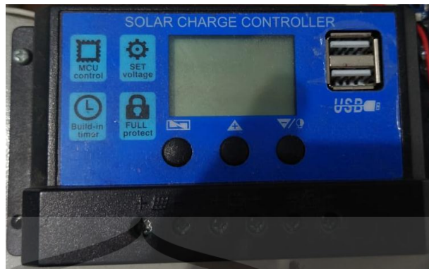
Gambar 2. 10 Solar Charger Controller
